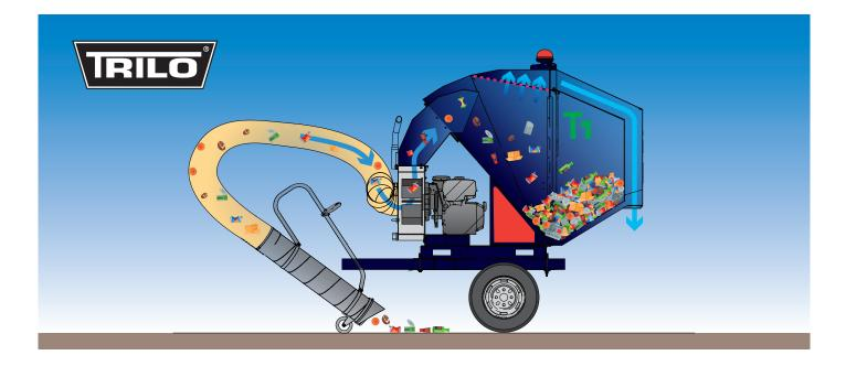
Impeller: Ø 400 mm – 4-blade Drive: Petrol engine - Honda GX340 8 kW Machine starting method: Pull cord Overall dimensions: (LxWxH): 209 x 150 x 160 cm Weight empty: 332 kg Load volume: 1.0 m<sup>3</sup> Suction hose: Ø 200 mm x 5 m (4 m flexible hose) Airflow: 180 m<sup>3</sup>/min
